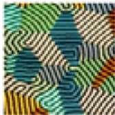
Magnetic domains garnet film 11 \mu\text{m} wide stripes
